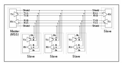
Figure 4-24. Example Four-Wire Mode Network
