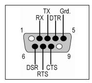
Figure 7-5: DB9 RS-232 Serial Connector
