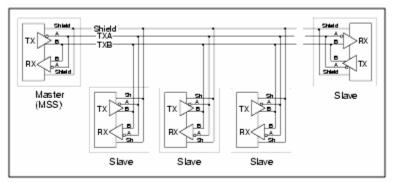
On a two-wire RS-485 network, the MSS must turn its transmitter on when it is ready to send data and then off a certain period of time after the data has been sent so that the
