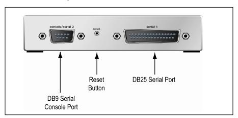
Figure 2-1: MSS-VIA Front Panel
