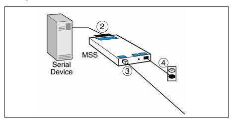
Figure 2-13: MSS Connected to Serial Device and Ethernet
