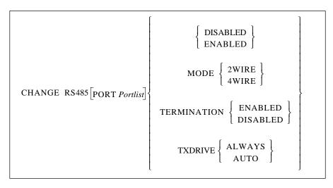
Enables RS-485 networking and configures the necessary RS-485 parameters on the MSS-VIA and the MSS4. RS-485 networking is explained in the *Configuration* chapter of your MSS installation guide.
