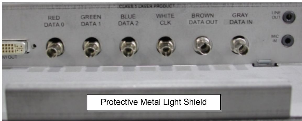
DVI Fiberlynx Transmitter, Fiber Optic ST connectors and Audio Jacks
