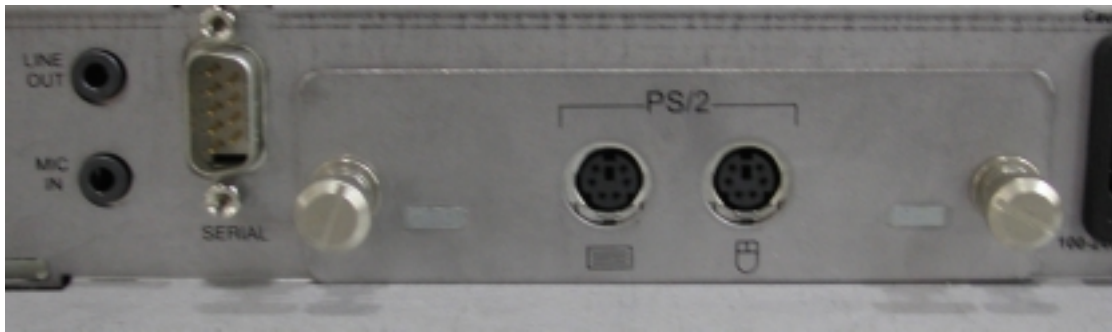
DVI Fiberlynx Receiver, Audio, Serial and PS/2 Connections
