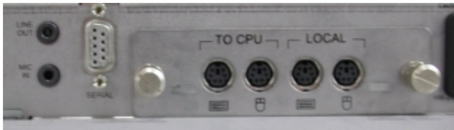
DVI Fiberlynx Transmitter: Audio, Serial and PS/2 Connections
