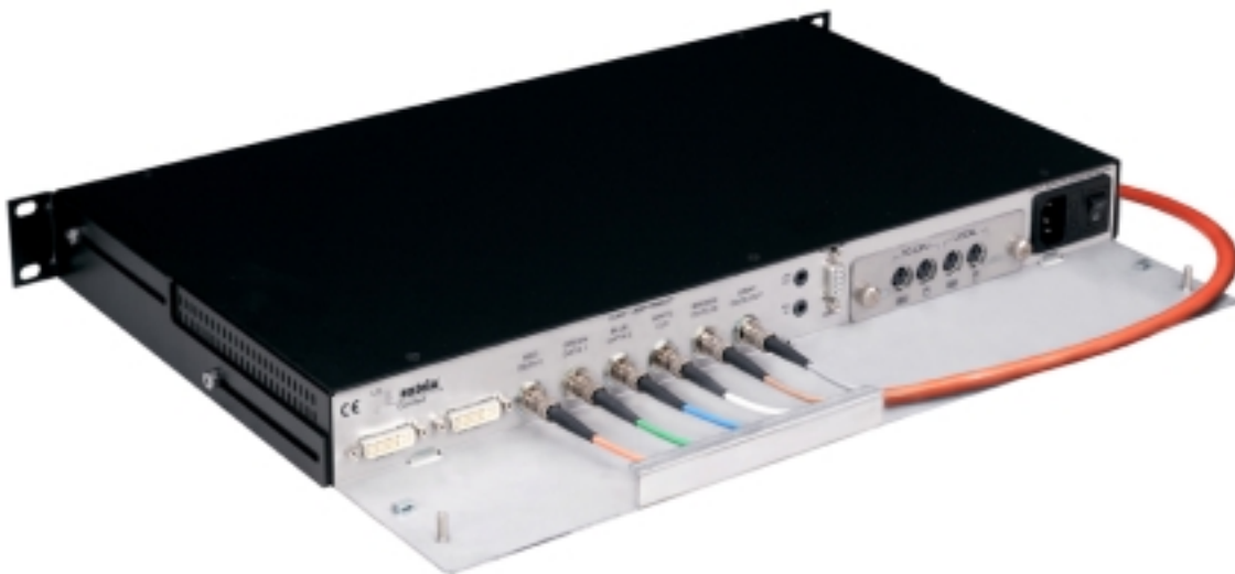
Rear of Transmitter unit, showing suggested Fiber Optic routing
