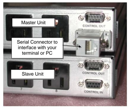
The **CONTROL OUT** Port is a DB9M Connector used to cascade **PCU8** boxes. A DB9M to DB9F Straight through cable is required.
